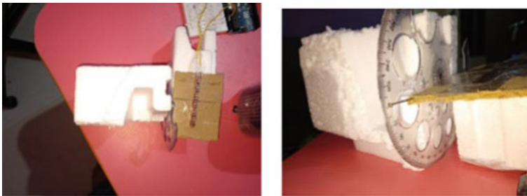
Fig. 3 Flexible force sensor calibration setup
