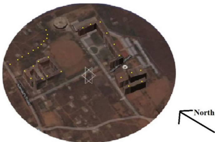
Fig. 14 Location of sample points on Vel Tech University campus for the placement of a 20 kW wind turbine at heights of 5 m and 25 m (Total: 30 points)
