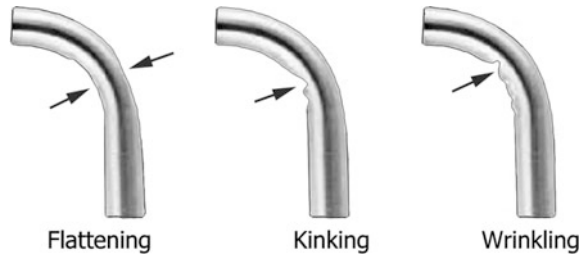
Fig. 1 Defects due to excess wall thinning
