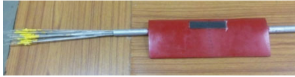
Fig. 3 Airfoil model with introduced roughed surface
