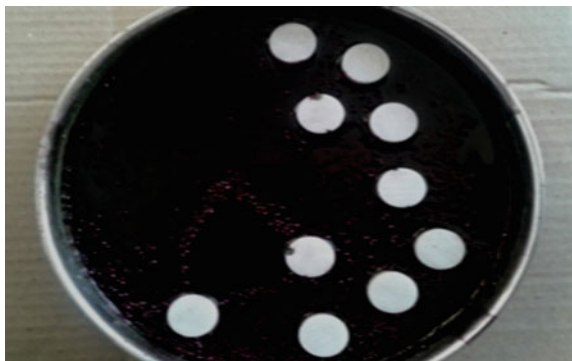
Fig. 2 Samples floating on the balls during dye penetration test
