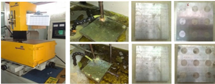
Fig. 1 EDM milling machine during machining of H12 tool steel with copper and copper–tungsten electrodes
